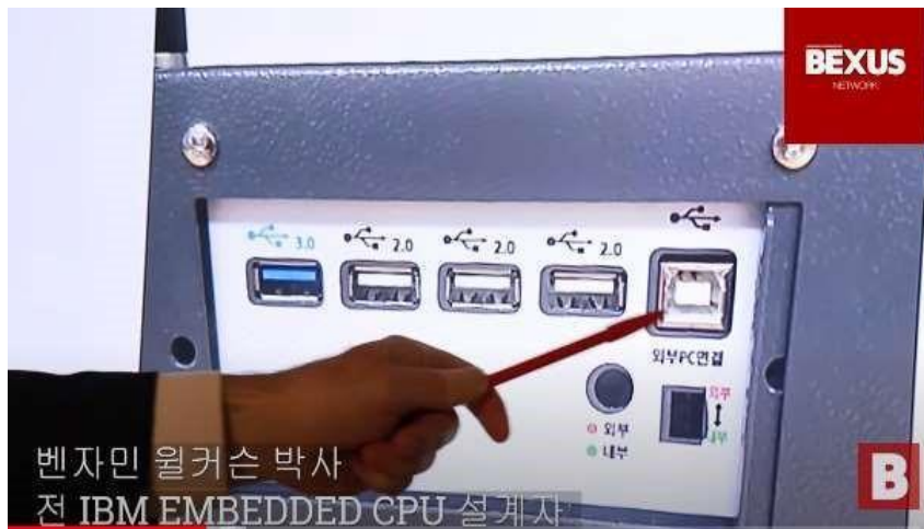
<Figure 2> USB ports in the ballot sorter
